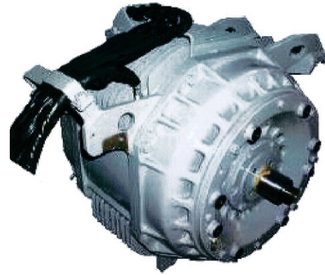
Fig. 14. Totally enclosed, self-cooled permanent magnet synchronous traction motor for narrow gauge EMU (1-h rated output 270 kW, grease lubrication) [16]
